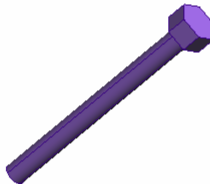
Figure 68. Completed 1/4 x 2.75" bolt.
